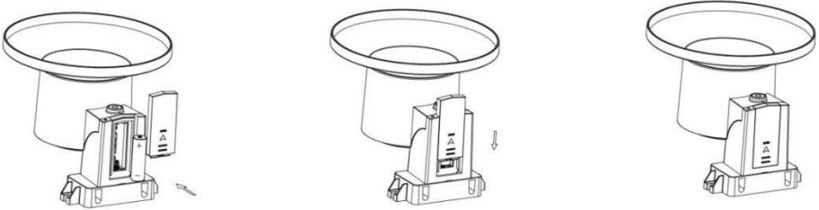
Figure 16: Rain gauge sensor battery installation diagram
