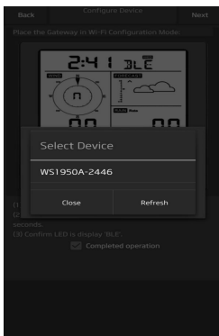
5) If you have more than one device they will all be listed. Select the device. The last four digits of device ID is same as its last four digits of MAC address. If cannot find your device ID, press refresh to update
