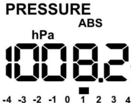
Pressure change tendency (updating every 60 second) is reflected by the scale indicator located under pressure display digits. Usually this is an indicator of weather change: when pressure is going in upward direction, it normally mean weather is getting better.
