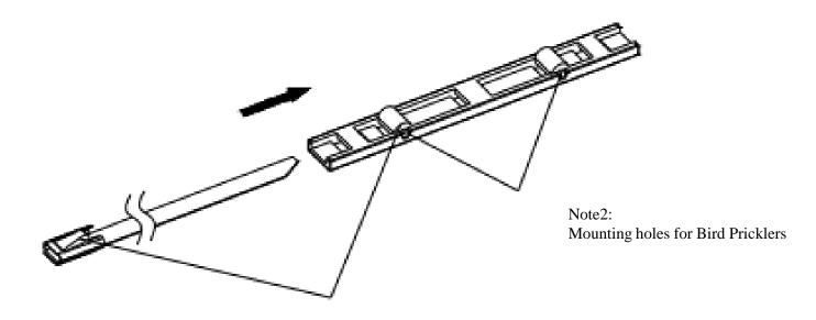
Note1: Please place the stainless steel cable tie and the rubber protrusion on the same surface
