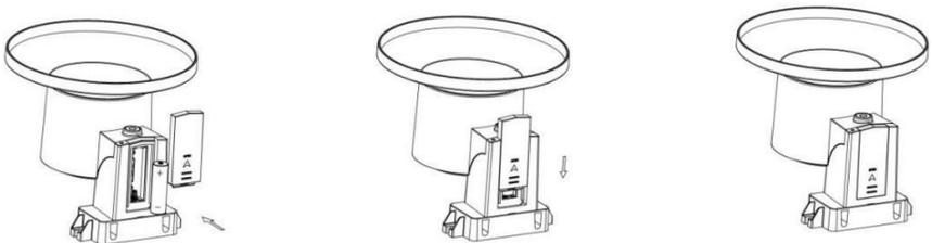
**Figure 16: Rain gauge sensor battery installation diagram**
