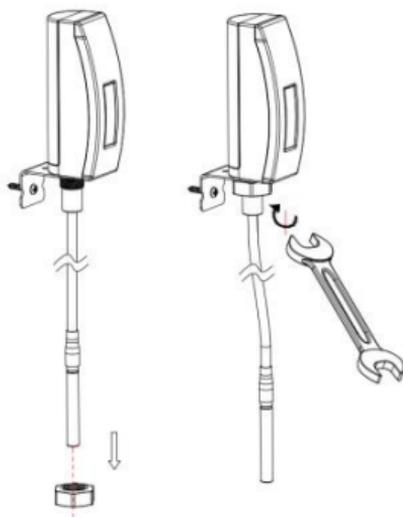
**Figure 3-2: Sensor mounting**
