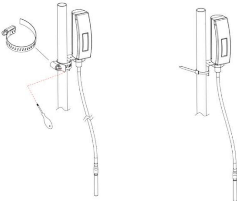
**Figure 4: Sensor mounting to pole**
