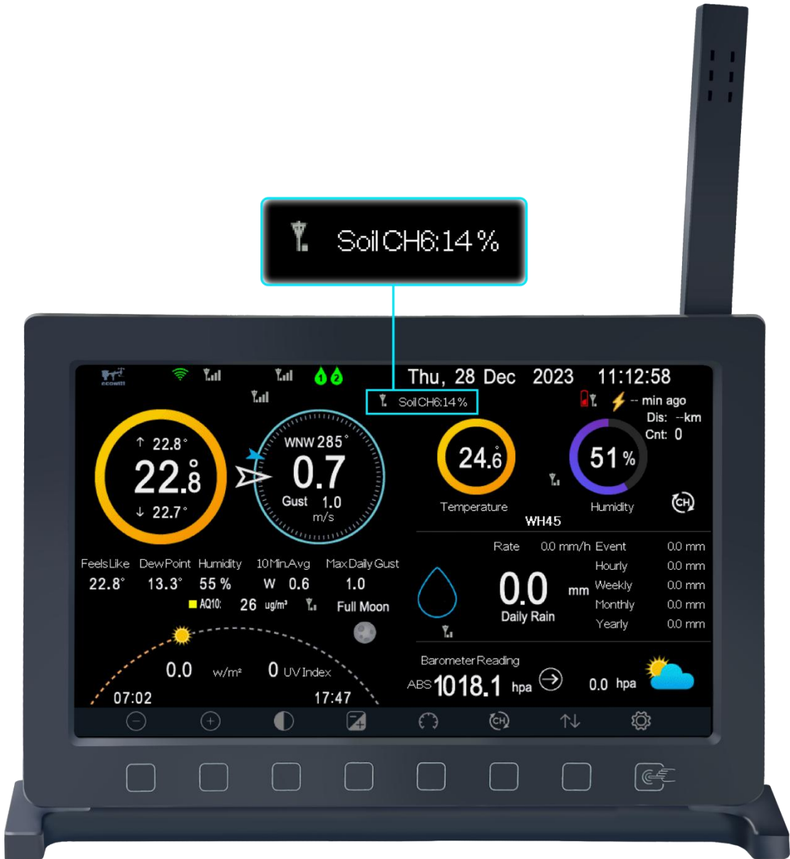
Figure 35: Data on Main Dashboard of HP2560
